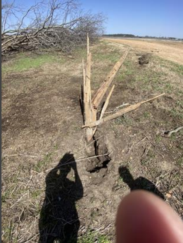
Power pole dragged ~18" through an embankment at Rolling Fork, MS, 24 Mar 2023; rated EF3
